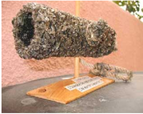
A Portland sampler that has been colonized by zebra mussels
